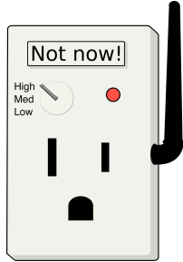
Figure 2: A possible “smart outlet” adapter to plug over an existing outlet. A three-way switch sets willingness to be shut off, which the “Not now!” button overrides. The outlet displays its mode with a multi-color LED, and communicates wirelessly with other outlets, appliances, and its meter box.
